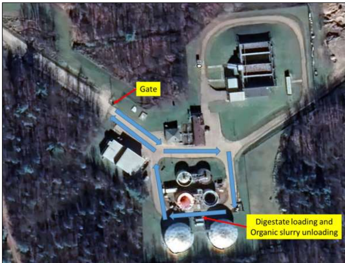
Figure 6-1: Truck routing diagram for digestate hauling trucks onsite.
